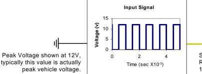
Square Wave Signal, at Recommended frequency: 500-1500Hz, (shown at 50% duty cycle)
